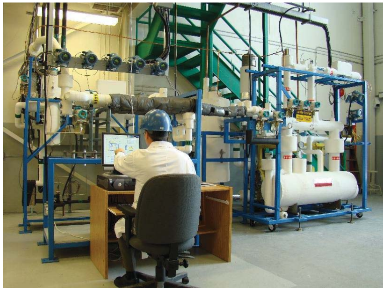
Figure 4-4: View of CanmetENERGY’s laboratory ejector test bench [Scott]
