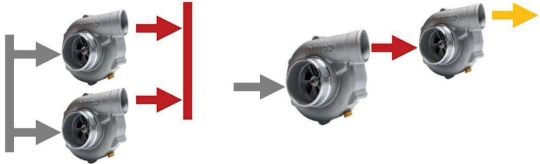
Figure 5-11: Compressor set up in parallel combined with serial coupling to match required capacity and pressure ratio
