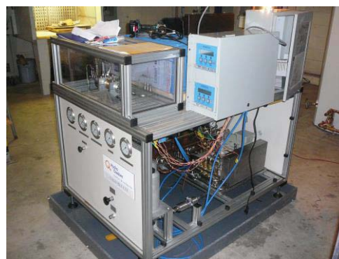
(a) (b) Figure 4-5: Experimental set-up of the ejector refrigeration system; (a) schematic diagram; (b) view of the laboratory prototype [Minea, 2011a; Minea, 2013]
