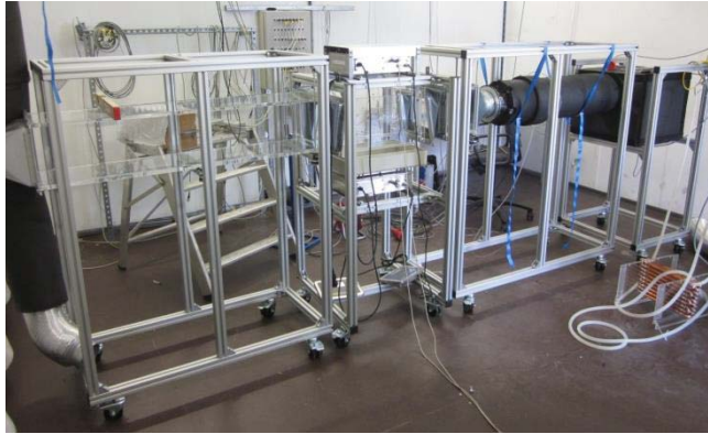
Figure 3-16: Test facility for experimental analysis of flue gas condensation @ AIT [Seichter et al., 2013]
