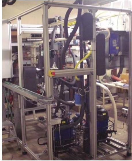
Figure 3-12: Picture of the absorption-/compression heat pump prototype @ IWT [Hannl & Rieberer, 2014]
