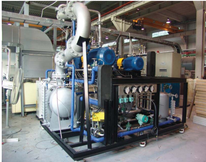
Figure 9-2: Prototype of a compression/absorption heat pump system
